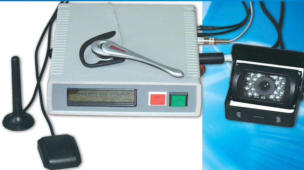
The onboard Controller of Monitoring of (BKM) is intended for satellite navigation and a wireless communication of GSM that allows to use (BKM) for control of location of object (vehicle), transfer of telemetric data (including object photos) and a wireless voice communication. Three fold reservation of the audiochannel. The patent application is submitted.
