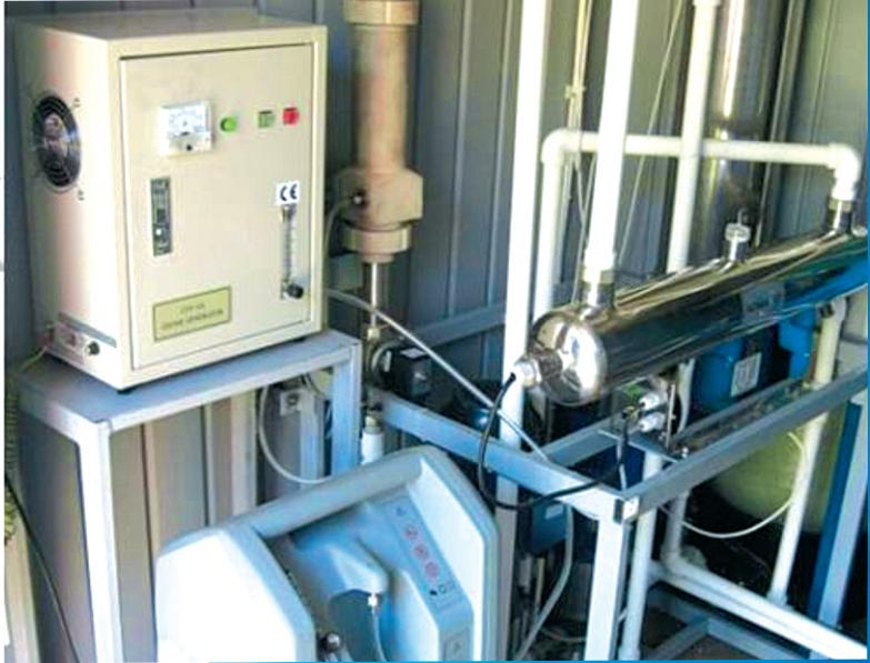
The (AFS-m) provides continuous water purification for the drinking and technical purposes at natural disasters, technogenic catastrophes and other emergency situations. The system can have various modifications and options (for example, portability, mobility, belonging to branch, productivity, existence of the automated analysis of quality, a set of algorithms of technological process). The patent application is submitted.
